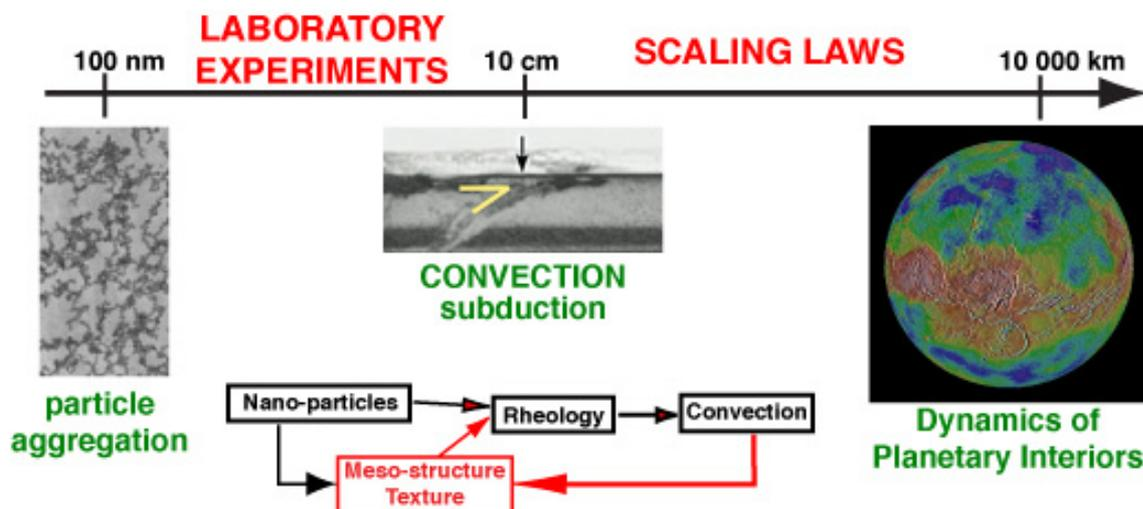
**Methods:** Aqueous colloidal silica suspensions will be used as a model system, where the nanoparticles size and volume fraction can be tuned to control rheology and induce aggregation. The work will combine fluid mechanics convection experiments, and state-of-the-art visualization and measurements techniques from nano- to cm-scales (neutron imagery, X-rays and neutrons diffraction, DLS, Raman and IR spectroscopy, rheology, thermography, LIF and PIV).
